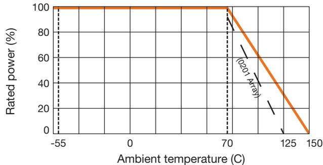
The resistors shall have a power rating based on continuous full-load operation at an ambient temperature of 70°C. For operation at ambient temperature in excess of 70°C, the load shall be derated in accordance with figure of Derating Curve.
